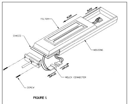
• Once out of the extrusion, the chassis and filter will come apart.
