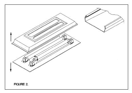
Carefully grasp the tube ends and twist one quarter turn until it works free (Fig. 2)
