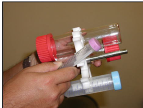
Installing the bottles and tubes
