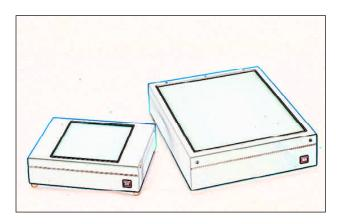
White Light Transilluminators offer the researcher cool white light through an evenly diffused glass surface. The plexiglass and glass combination is permanently sealed into the unit - double sealed safety fused for durability. Excellent for viewing coomassie blue stained gels as well as autoradiographs, X-Rays, and microtiter plates. The TW-26 is designed for use with 8 x 10" film sizes; the TW-43 with 14 x 17" film sizes.
